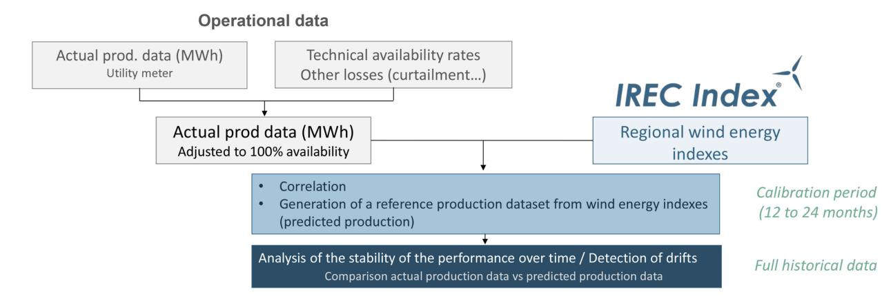
If availability rates are consistent in time (method of calculation and types of downtimes taken into account), the deviation between the actual production and the predicted production (reference production issued from IREC Indexes) should reflect an evolution of the production capacity of the wind farm (i.e. its performance) such as:
