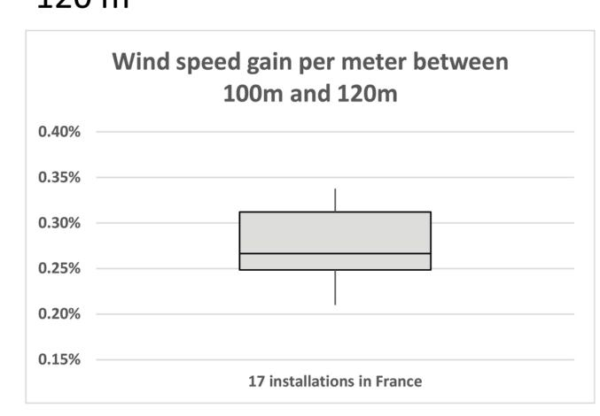
The wind speed gain per meter  $(WS_{gain\_m})$  between 100 m and 120 m is relatively stable for all the installations (variation between 0.21% and 0.31%). In this method, a median of 0.27% wind speed gain per meter was considered for all projects.
