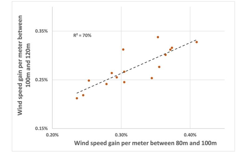
A linear regression (Y = AX + B) between the  $WS_{gain\_m}$  established between 120 m and 100 m and the one established between 100 m and 80 m was considered.
