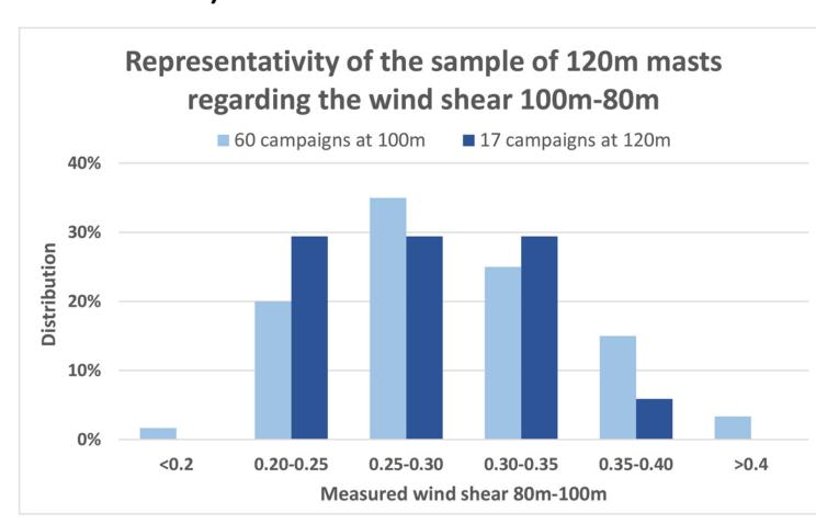
In order to generalize the results on a larger scale, the wind shears between 80 m and 100 m were compared for these 17 installations and for 60 installations of 100 m.
